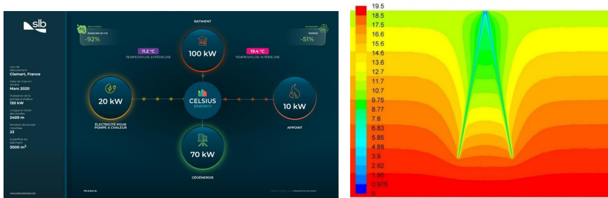
Figure 2: layout of a Geoenery Management System dashboard (left) and temperature distribution modelling using a bespoke finite-volume simulator (right)
